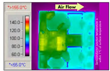
Figure 6: Thermal plot of converter at 18 amp load current (217 Watts) with 55°C air flowing at the rate of 200 LFM. Air is flowing across the converter from input to output (nominal input voltage).
