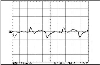
Figure 16: Output Voltage Ripple at nominal input voltage and rated load current (20 mV/div). Load capacitance: 1µF ceramic capacitor and 15µF tantalum capacitor. Bandwidth: 20 MHz. (See Figure 13)
