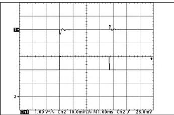
Figure 12: Output voltage response to step-change in load current (50%-75%-50% of Iout(max):  $dI/dt = 5A/\mu s$ ). Load cap:  $480\mu F$ ,  $15 \, m\Omega$  ESR tantalum and  $1\mu F$  ceramic. Top trace: Vout (1V/div), Bottom trace: Iout (5A/div).
