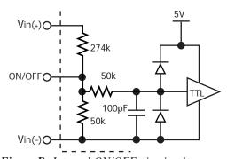
Figure B: Internal ON/OFF pin circuitry
