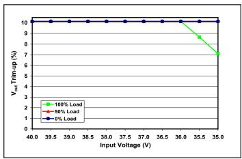
Figure 23: Achieveable trim-up percentage vs. input voltage. at output loads of 0%, 50% and full load.
