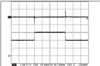
Figure 11: Output voltage response to step-change in load current (50%-75%-50% of lout(max);  $dI/dt = 0.1A/\mu s$ ). Load cap:  $15\mu F$ , 450 mW ESR tantalum and  $1\mu F$  ceramic. Top trace: Vout (IV/div), Bottom trace: lout (5A/div).
